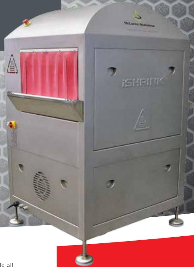
Running at 16-21Kwh, in typical use, it is considerably more efficient than other tunnels in use today. It uses a unique water heating and recovery system to achieve supreme shrink performance.
